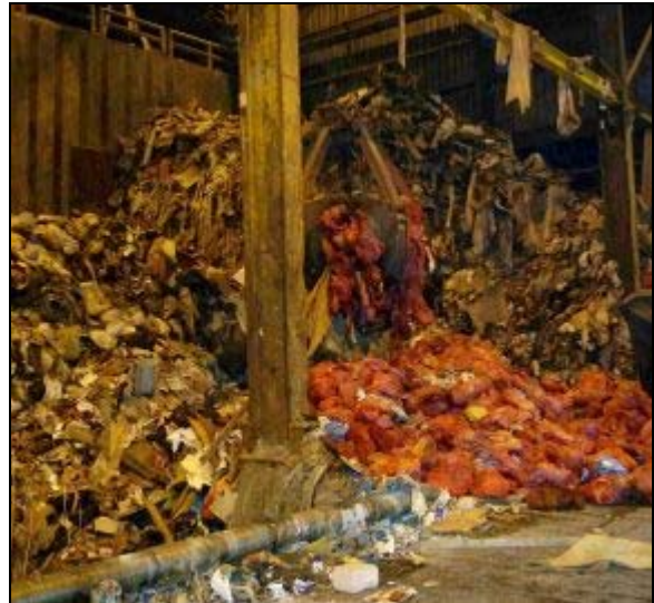
Solid waste being readied for incineration and conversion to steam energy at Dutchess County's waste-to-energy facility.
