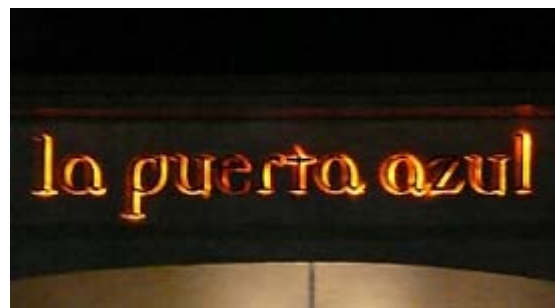
The subtle glow around the backlit letters provides enhanced readability without creating glare.
